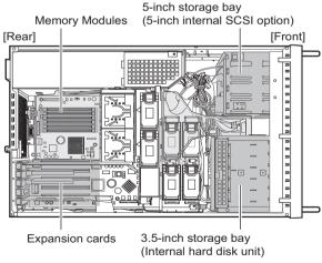
After installing internal options, check that the order and location of installation are correct and cables are correctly attached.
